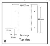
Position the base into the recess with its front edge as far forward as the adjoining plinth line will allow.
